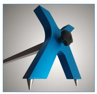
Figure 32 Alignment jig end-piece
