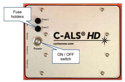
Figure 10 Surface unit internal panel
