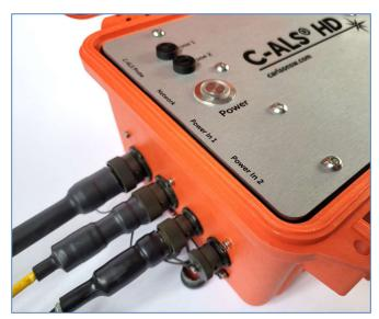
Figure 9 Surface unit connections from left to right: main C-ALS cable, data cable, one power cable and a spare connector for an additional power cable
