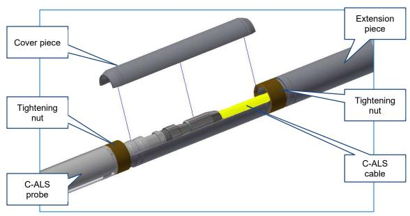
Figure 6 Attaching the cover piece
