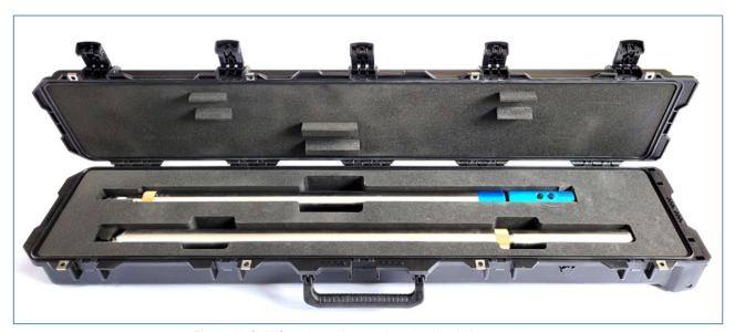
Figure 29 C-ALS probe and extension piece in their transit case
