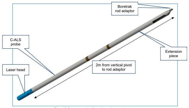
Figure 7 Complete unit with probe and extension piece
