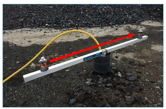
Figure 36 CALS probe in a borehole on a vertical alignment jig - showing direction of reference azimuth
