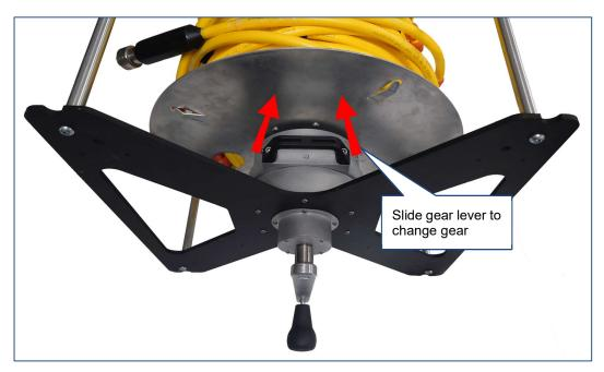
Figure 17 Sliding the gear lever to change to a lower gear
