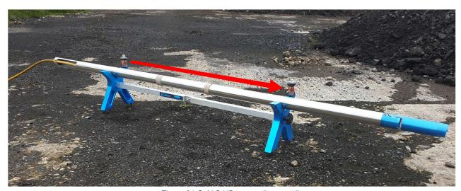
Figure 31 C-ALS HD on an alignment jig
